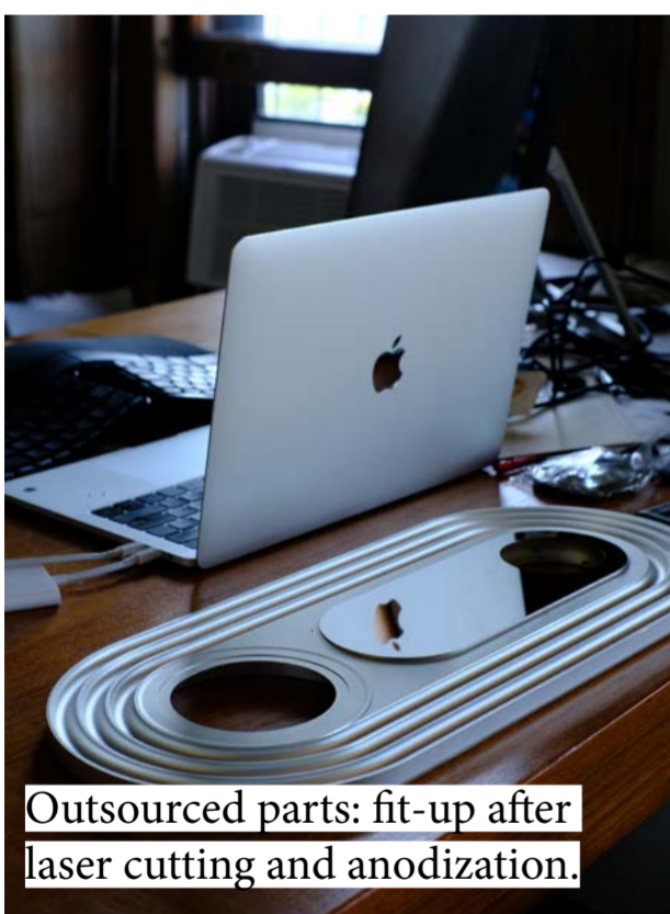
Functional prototype: half-height base reduces machining cost and leaves underside open for prototyping componentry.
