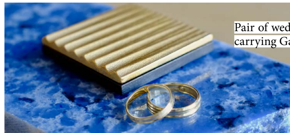
Presentation box constructed from two parts, produced in iron via SLS (selective laser sintering) and blackened/plated to achieve finished colors.
